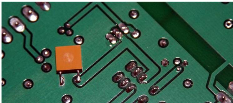
In later revisions of the SWCTRL board, this CK06 ceramic snubber capacitor will be normally mounted on the component side of the board.
