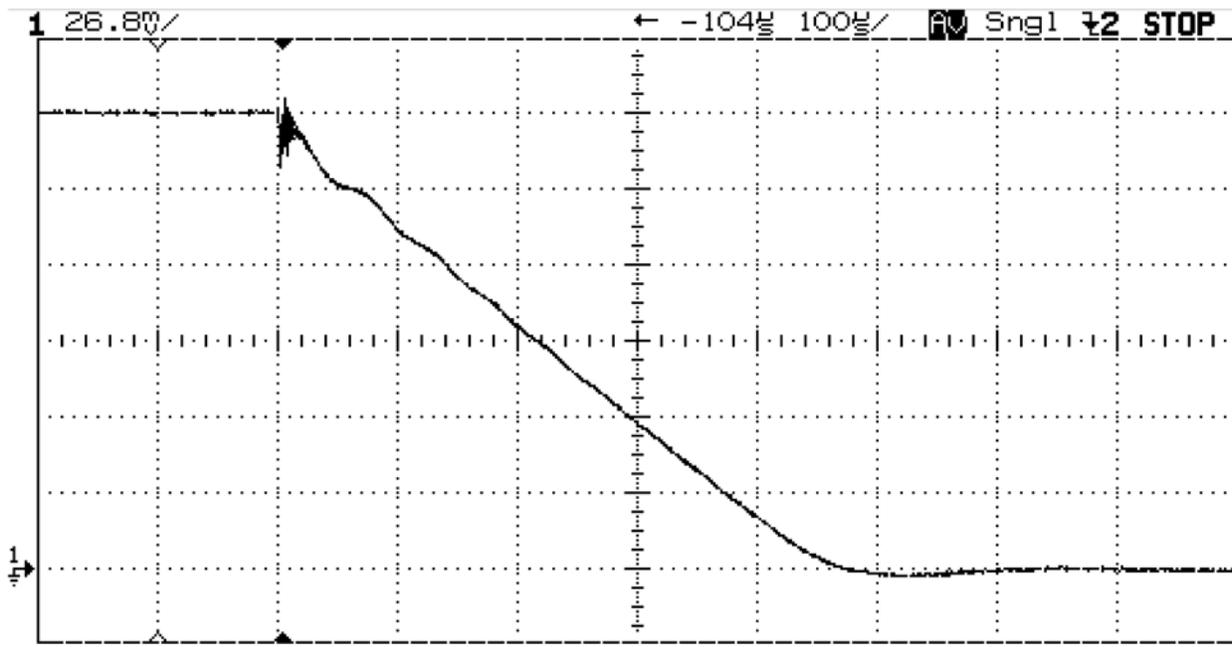
The oscillogram of powered coil current versus time shows the resulting linear ramp and final roll out from the L/R secondary dump resistor discharge. This current discharge oscillogram was based on a voltage measurement across a 0.1 ohm resistor temporarily placed in series with the “low side” lead of the powered coil cable wire. The oscilloscope was momentarily floated from AC mains ground so that the scope probe ground probe could be at a voltage different from chassis ground.
