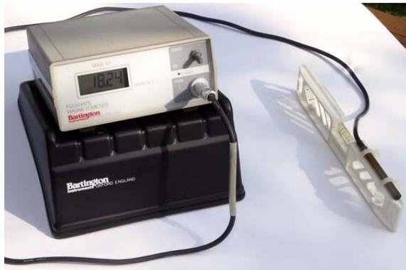
Bartington MAG-01 fluxgate magnetometer<sup>7</sup>, sensor mounted on a plastic level
